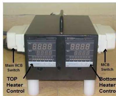
Fig.8 Profile based Temperature Controller with MCB and RCB switches
