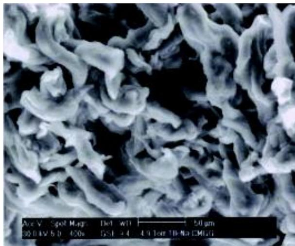
**Figure 10 :** Scanning Electron Micrograph of Na-PCMG (DS = 0.497) (400X)
