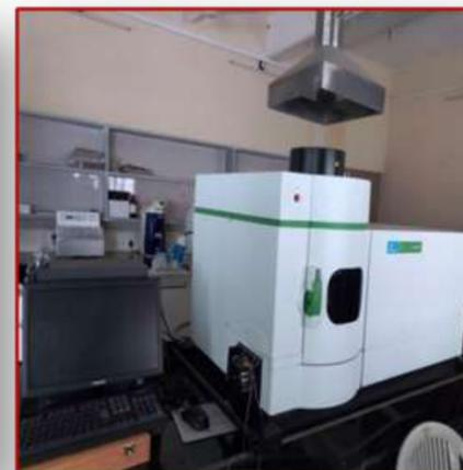
**INDUCTIVE COUPLED PLASMA OPTICAL EMISSION SPECTROSCOPY**
