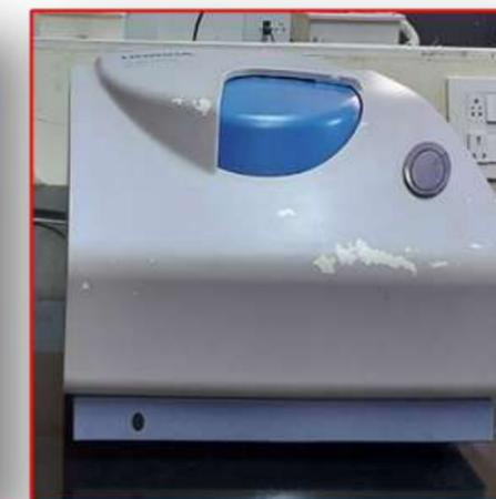
**PARTICLE SIZE ANALYZER WITH ZETA POTENTIAL MEASURING SYSTEM**
