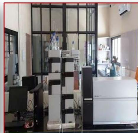
**TRIPLE QUADRUPOLE HIGH PERFORMANCE LIQUID CHROMATOGRAPHY (LC-MS/MS)**
