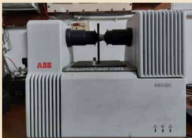
IR Spectrometer MB3000 ABB 500 to 4000 \text{cm}^{-1}
