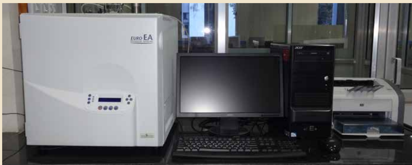
Elemental Analyser (CHNS) EURO-EA-3000, EURO-vector, Temp. upto 1100°C
