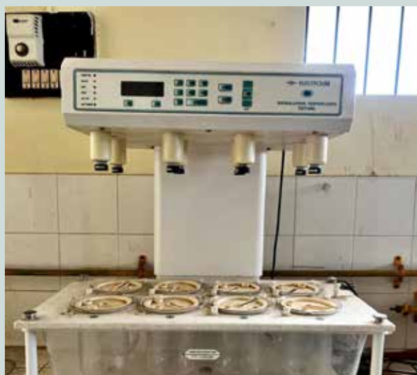
Dissolution Test Apparatus TDT-08, Electrolab
