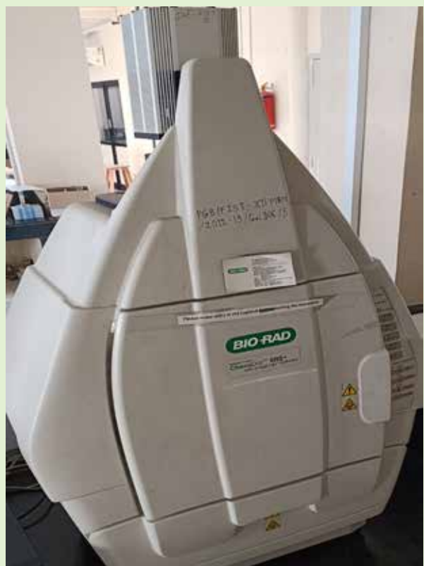
Gel Documentation System Biorad Chemi Doc Xrs+ Gel imaging in UV and Visible range
