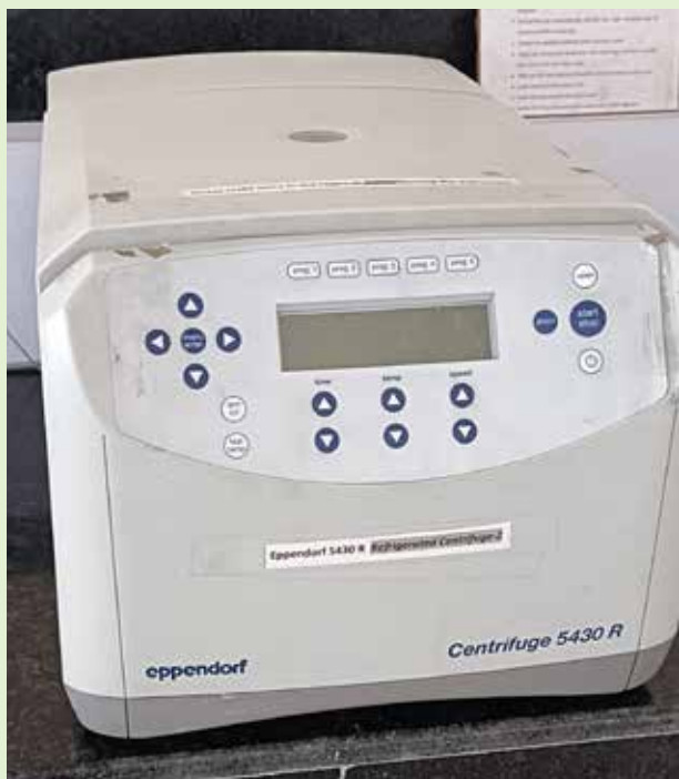
Refrigerated Centrifuges Eppendorf 5430R ,SIGMA 3K30, 30K-RPM, 4°C TEMP
