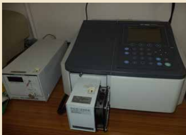
UV-Visible Spectrometer SHIMADZU, Double Beam, (200 to 800 nm Wavelength) absorbance 0 - 4.
