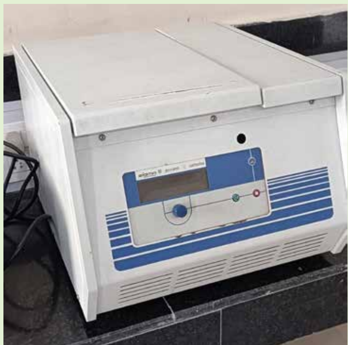
Refrigerated Centrifuges Eppendorf 5430R ,SIGMA 3K30, 30K-RPM, 4°C TEMP
