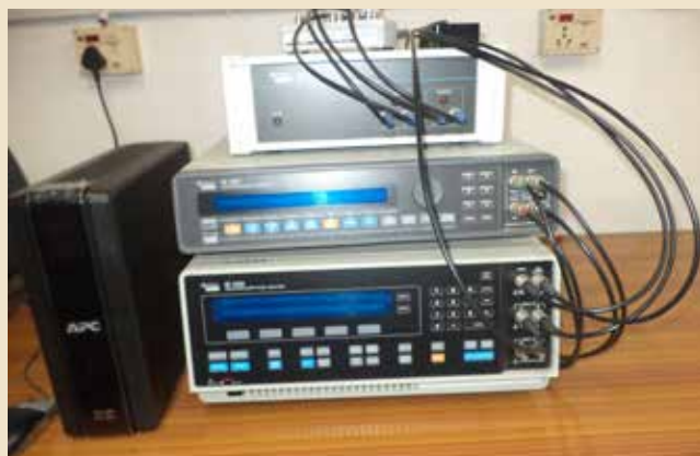
Solartron Electrochemical workstation SI-1260, SI-1296 and SI-1287 Solartron, UK, 1Hz to 1.2 MHz frequency sweep, Electrochemical workstation with Electrical study
