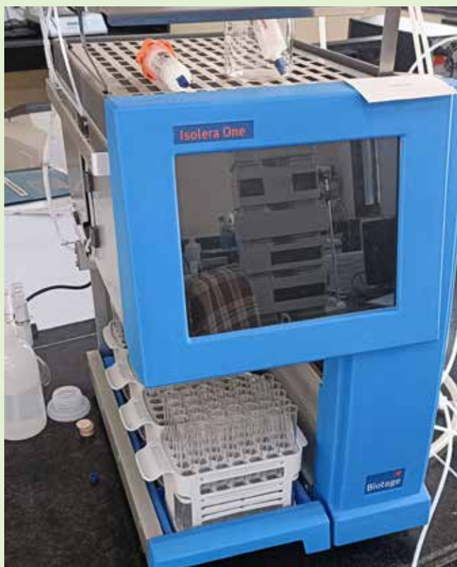
Flash Purification System BIOTAGE ISOLERA 1, PDA DETECTOR
