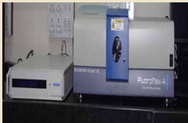
Fluoromax-4 Spectrophotometer FLUROMAX 4CP-TCSPC, Horiba Jobin Vira Edison, USA, Excitation and emission analysis 250-800 nm
