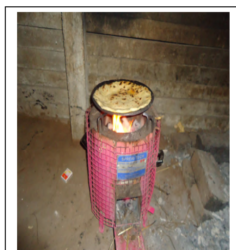
Figure 3.4b Biomass cook stove-Air insulated -Side feeding (in use)
