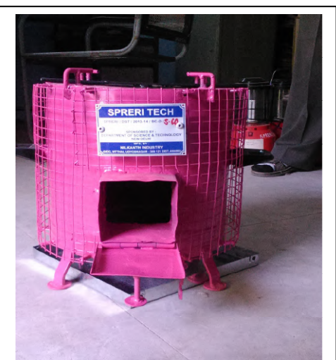
Figure 3.4a Biomass cook stove-Air insulated -Side feeding
