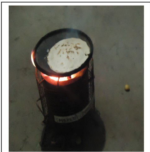
Figure 3.3b Biomass cook stove-Air insulated -Top feeding (in use)
