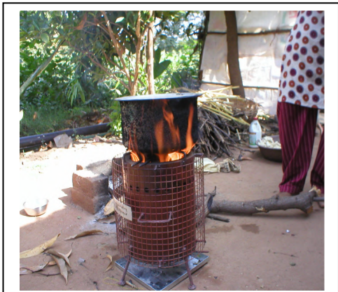
Figure 3.2 Ceramic Liner Cook Stove (in use)
