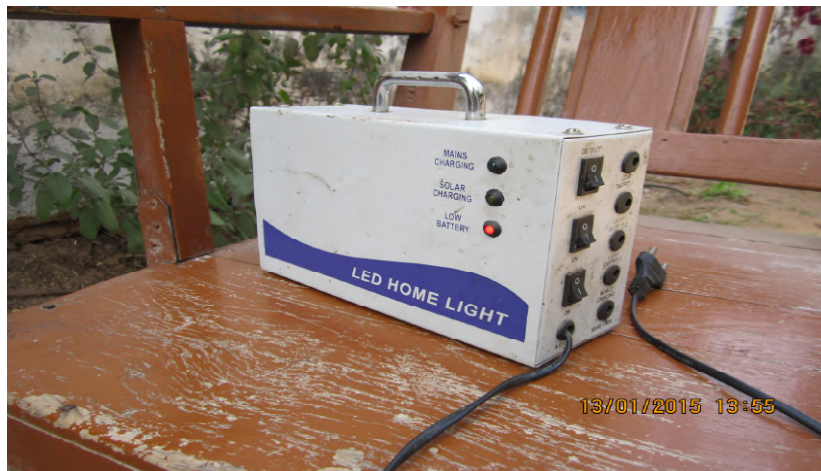
Figure 3.11 . Battery set up for Solar Home Light System (HLS)
